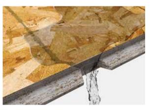
All LP® TopNotch® OSB sub-flooring products feature the RainChannel $^{\text{TM}}$  self-draining notch system, which allows water to drain quickly from the surface. Combined with a moisture-resistant edge seal, the RainChannel system helps fight moisture absorption and edge swell, reducing the need for sanding.
